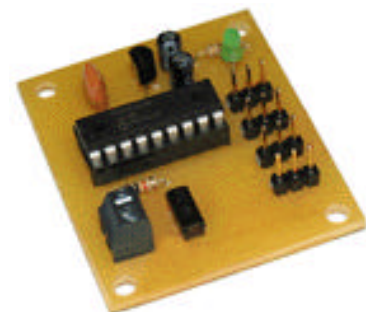
Duo Input 1-Ch Servo Switch over (Servo Control by Manual and RF Control)
