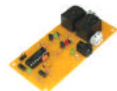
R/C Motor Controller (BPE # RCR-8600)
