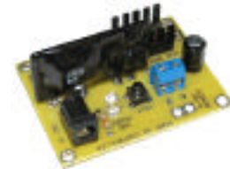
Air / Pump Switch (BPE # MWC-0344)
