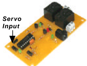
Servo to 10 Amp DC Motor Controller
