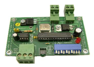
A single channel PWM Led Driver Board can be used to control a single Led light source from a DMX control signal.
