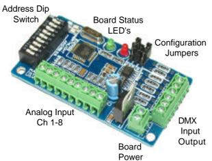
The analog voltage (0-10 Vdc) is converted to 255 discrete DMX levels (0-255). The controller can be used to upgrade older 0-10 volt analog light ing consoles, or add your own switches and potentiometers to create custom controls for lighting, home or building automation and animatronics applications.
