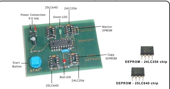
The **EEPROM Rom Copy** board provides a quick and convenient means of duplicating the serial EEPROM's used in the Puppeteer, Animate and Wizard family of control boards.
