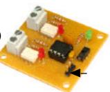
Servo to Duo 1Amp or Single 2Amp Solid State Relay
