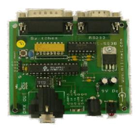
The TX512 transmitter is a full speed serial to DMX transmitter. The module will generate up to 512 DMX channels and accepts serial commands and data via a standard 9600/19200 baud 8-N-1 RS232 serial connection- eq PC.
