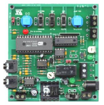
Wizard - VIII Board is pre-assembled and tested. Regulated 9 Volt dc power supply @ 0.5 Amp power supply required.
