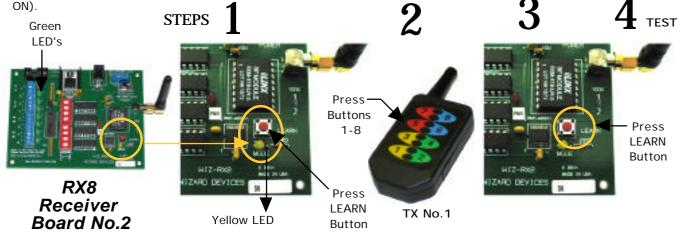
Single RF Transmitter and Multiple Receivers
