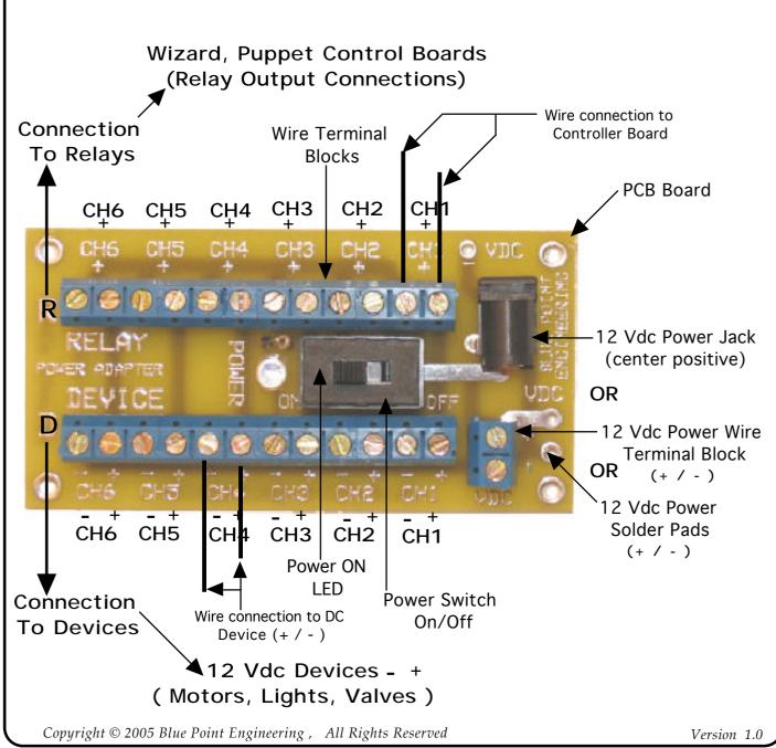
Module is rated for 5 Amp loads at 12 Vdc.
