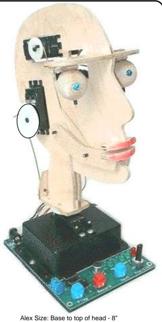
Nose to back of head - 6" Control Board Size: 5" L x 4-3/16" W Power Requirements: 9 Volts dc @ 2 Amp.
