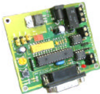
Board Size: 2-3/4" L x 3-5/16" W x 1/2" H Power Requirements: Regulated 5 VDC @ 2.5 Amp supply
