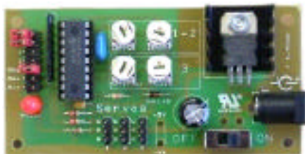
Board Size: 3-1/2" L x 1-3/8" W x 1/2" H Power Requirements: Regulated 9 VDC @ 2 Amp supply
