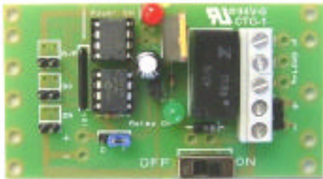
Board Size: 3" L x 1-1/2" W x 1/2" H Power Requirements: Regulated 9 VDC @ 0.5 Amp supply
