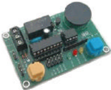
Board Size: 2-1/2" L x 1-1/2" W x 5/8" H Power Requirements: Regulated 5 VDC @ 1 Amp supply
