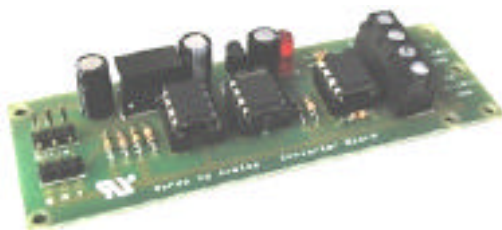
Board Size: 3-5/8" L x 1-1/4" W x 3/4" H Power Output: 10 mA / adjustable 0-10 Vdc
