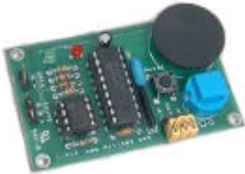
Board Size: 2-1/2" L x 1-1/2" W x 5/8" H Power Requirements: Regulated 5 VDC @ 1 Amp supply
