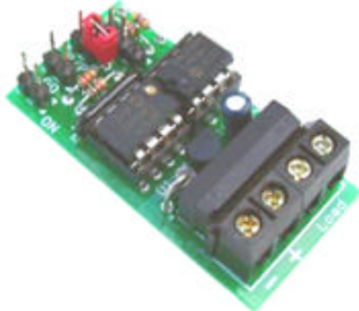
Board Size: 1-7/8" L x 1" W x 1/2" H Power Requirements: Regulated 9 VDC @ 0.5 Amp supply
