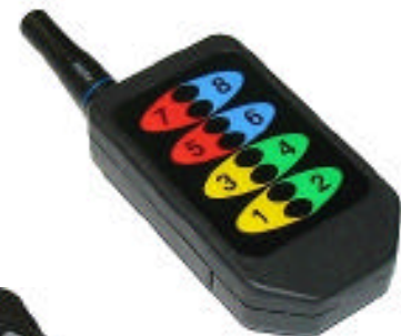
Long Range Transmitte (TX)
